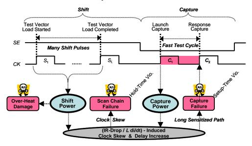
Figure 1. Impact of Test Power in LOC-Based At-Speed Scan Testing
